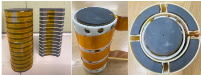
Fig. 10: Center post and one fourth of the outer shell stacked using core pieces and spacer material (left). Copper foil wrapped around center post through the PTFE support structure (center). Top view of the center post, outer shell and copper winding held together through the ultem support structure (right)
