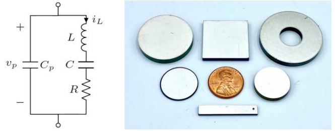
Fig. 1. Butterworth-Van Dyke circuit model [6-8] and example PRs.
