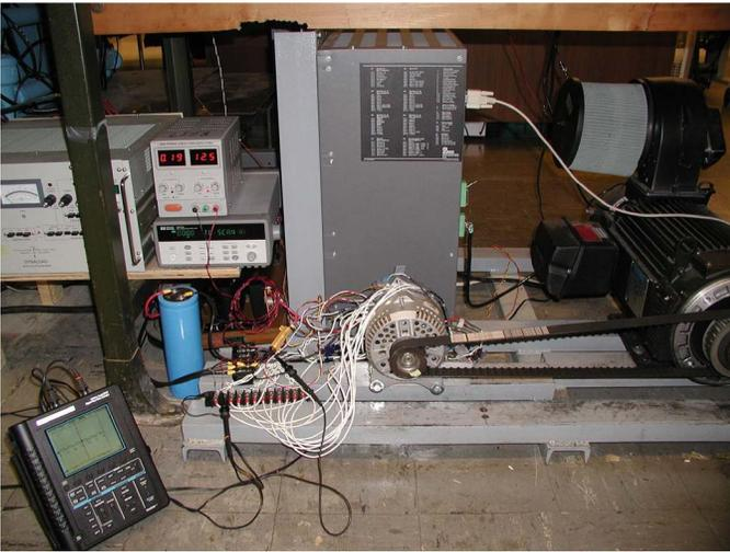
Figure 8 The experimental setup used to test the prototype system. The system enables measurement of voltages, currents, and temperatures across a wide range of drive and load conditions. Details of the experimental apparatus and methods may be found in [26].
