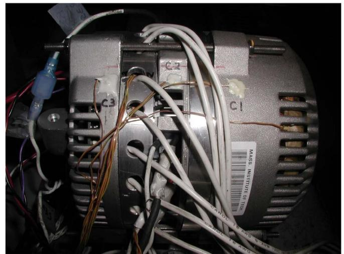
Figure 7 The prototype 4-cell alternator. The 42 V alternator and power electronics are completely integrated. Numerous voltages and temperatures are brought out for evaluation purposes.
