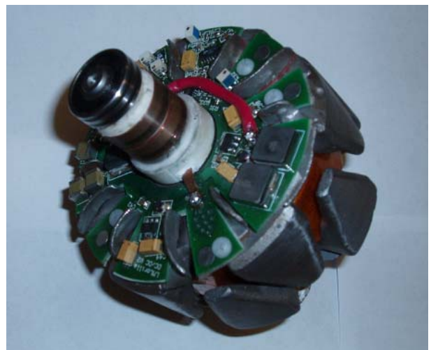
Figure 4: Foil-wound rotor and rotating dc-dc converter [17,18].
