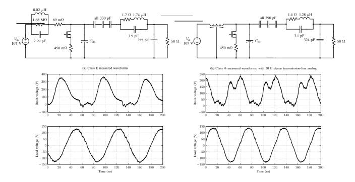
Fig. 8: Schematics and measured waveforms of the Class E and Class  $\Phi$  inverters
