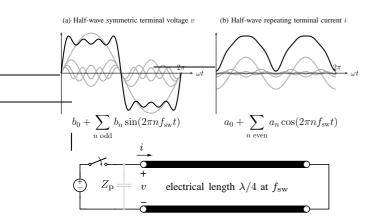
Fig. 2: Input impedance (left) of a line of length  $\ell$  terminated in a short circuit. When excited periodically at a frequency equal to the principle quarter-wave resonance, the line enforces odd- and even-harmonic symmetries in voltage and current, respectively.
