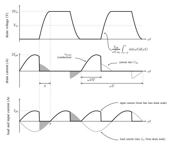
Fig. 3: Waveform symmetries (left) imposed by the  $\lambda/4$ -wave transmission line, and idealized waveforms (right) of the Class  $\Phi$  inverter built around it.
