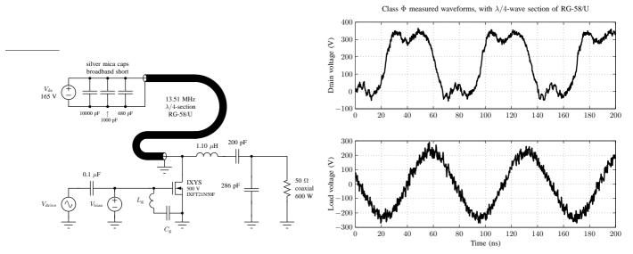
Fig. 5: Multi-resonant converter constructed with a length of RG-58/U coaxial line.
