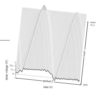
Fig. 4: Waveform symmetries (left) imposed by the  $\lambda/4$ -wave transmission line, and idealized waveforms (right) of the Class  $\Phi$  inverter built around it.
