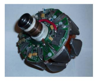
Fig. 4. Pressed rotor claws with foil field winding and rotating dc-dc converter.
