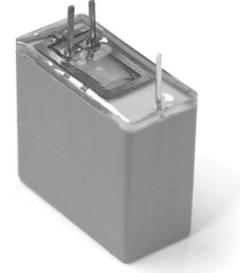
Fig. 25. Photograph of a completed 1.0  $\mu\text{F}$  integrated filter element with inductance cancellation. The resulting package height is 1.2 mm taller than the original capacitor casing.
