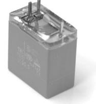
Fig. 21. Photograph of a completed 330 nF integrated filter element with inductance cancellation. The resulting package height is 1.75 mm taller than the original capacitor casing.
