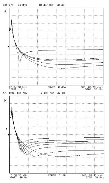
Fig. 9. Highest curve in both (a) and (b) represents the performance of a capacitor without any inductance cancellation in the test setup of Fig. 7. The curves in (a) are the results with center-tapped transformers having mutual inductances between 6 nH and 26 nH at intervals of 4 nH each. (b) The results of having a mutual inductance that is too large; these curves are the results with transformers having mutual inductances between 26 nH and 32 nH with intervals of 2 nH.
