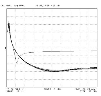
Fig. 10. Repeatability curves. The higher curve is a capacitor alone (no cancellation). The lower curves are results with six nominally identical circuits incorporating printed cancellation windings. Note that the curves are all within 3 dB of each other.
