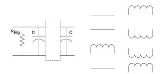
Fig. 16. EMI filter under test. The box can be replaced by any of the four connections shown. The filter can also use capacitors with or without inductance cancellation.
