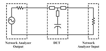
Fig. 7. Experimental setup for evaluating filters and components incorporating an Agilent 4395A network analyzer. The device under test (DUT) comprises of a filter capacitor and a printed circuit board inductance cancellation transformer with their interconnects.
