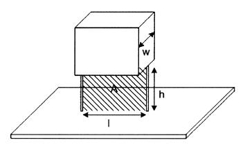
Fig. 6. Parasitic inductance created by lifting the capacitor off the board can be approximated using l, h, w, and  $\mu_0$ .
