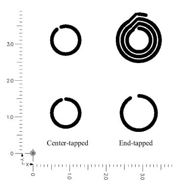
Fig. 5. Examples of center-tapped and end-tapped transformers. These are the transformers used for Table I. The left column has the top and bottom-side traces of the center-tapped transformer as viewed from the top side. The right column has the top and bottom-side traces of the end-tapped transformer as viewed from the top side. Length marks are in inches.
