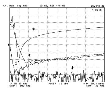
Fig. 18. Results of the EMI Filter test. Signal a is the performance of two normal capacitors. Signal b is the performance of two capacitors with inductance cancellation. Signal c is the performance of a normal capacitor with a single inductor in the series path. Signal d is the noise floor.
