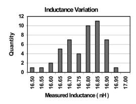
Fig. 4. Histogram of the parasitic inductances found for Beyschlag Centrallab 2222 338 24 224 X-type capacitors ( $0.22 \ \mu$ F, 275 Vac). The average value is 16.81 nH, with a standard deviation of 112 pH.
