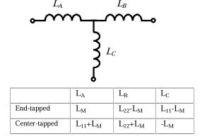
Fig. 2. Equivalent circuit model for the configurations of Fig. 1.
