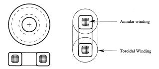
Fig. 19. Structural diagram of a cross-field reactor. The magnetic core is wound with two windings (an annular coil and a toroidal coil) that are not coupled in the usual sense. Current in one winding modulates the inductance seen at the other winding.
