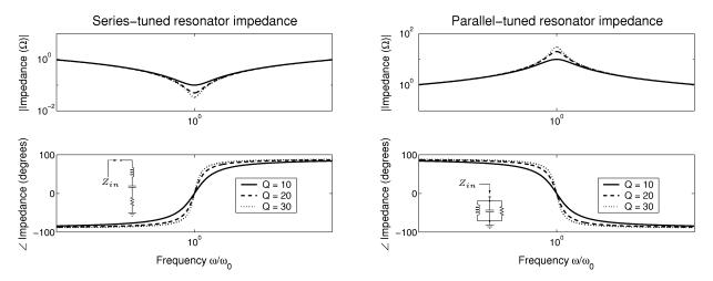
Fig. 1. Frequency response of second-order tuned circuits, normalized to the natural frequency  $\omega_n = 1/\sqrt{LC}$ . The impedance magnitude at a single frequency can indicate proximity to resonance (with calibration) but not whether resonance lies above or below the stimulus frequency. The impedance phase, however, increases or decreases monotonically, and its difference from  $0^{\circ}$  is an error signal indicating the distance and direction to resonance.
