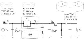
Fig. 11. Comparison of the core sizes for the input filter of a 300 W buck converter. The small film capacitors did not contribute significantly to the filter volume
