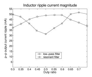
Fig. 15. Comparison of the peak-peak ripple performance of the single-inductor and resonant input filters.
