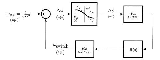
Fig. 7. Linearized model for the phase-sensing tuning system in lock.
