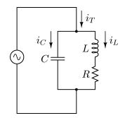
Fig. 5. "Almost-parallel" resonant circuit in which inductor loss dominates.
