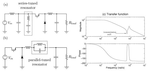
Fig. 2. Examples of a resonant filters in a buck converter. (a) The series-tuned leg provides a low-impedance current path (i.e. high attenuation) at a discrete frequency. (b) The parallel-tuned resonator presents a high impedance to switching ripple at a discrete frequency. (c) Transfer function: switch drain current to input current or switch source voltage to output voltage.
