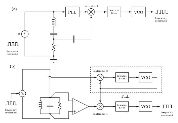
Fig. 3. Block diagram of the phase-lock tuning system for series and parallel resonators. In each case, equivalent tuning controls can be implemented by switching the sensing connections, e.g., by phase-locking to the tank voltage rather than the tank current in the lower diagram. Such an exchange, however, would not take advantage of phase-lock loop's ability to cleanly extract the fundamental component from the signal most dominated by harmonics.
