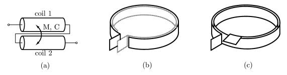
Fig. 18. Hybrid inductive-capacitive elements that exhibit resonances: (a) and (c) self-resonant inductors with large inter-turn or inter-coil capacitance and (b) schematic depiction of a resonant foil capacitor, similar to a typical film capacitor without extended-foil contacts.
