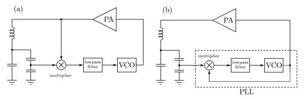
Fig. 4. Alternative resonant-excitation topologies. The PA blocks are power transimpedance amplifiers with current-drive outputs (such as switching converters). The capacitive dividers sense the current driving the series-tuned resonators (far left in each subfigure) with a 90° phase shift.
