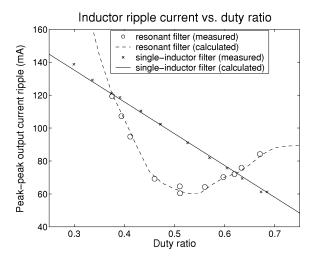
Fig. 12. Comparison of the peak-peak inductor ripple current performance of the single-inductor and resonant power stages.
