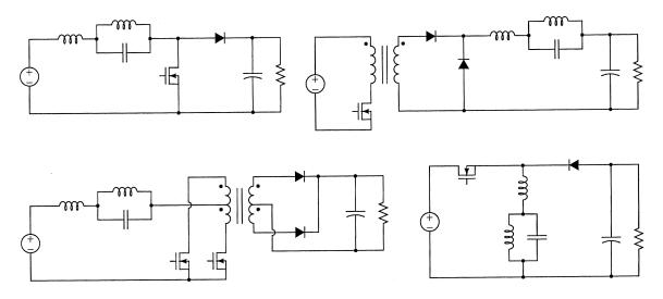
Fig. 17. Parallel-tuned resonant filters can be applied to the power stages of most major PWM switching-converter topologies.
