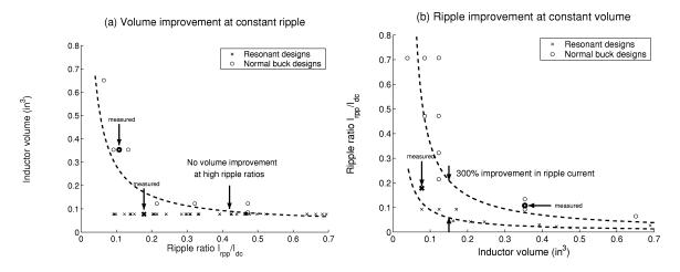
Fig. 13. Comparison of resonant and nonresonant buck converter magnetics designs. (a) Presentation comparing volume over peak-peak inductor current levels, including high ripple ratios which favor nonresonant designs. (b) Presentation comparing ripple ratio when resonant and nonresonant magnetics are allowed to fill the same volume.
