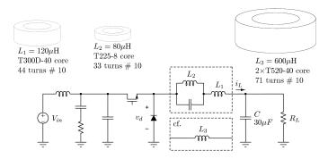
Fig. 10. Comparison of the core sizes for the power stage of a 300 W buck converter.
