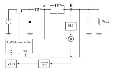
Fig. 9. Block diagram of phase-lock tuning system used to align a buck converter's switching frequency to the maximum-impedance resonance of its output filter. A ground-referenced voltage measurement is made at point A, from which the AC voltage across the tank is determined. The resonator current is measured at point B.
