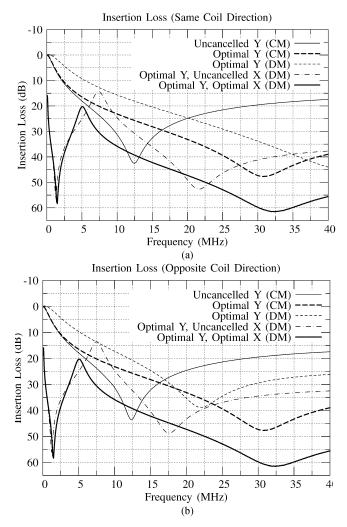
Fig. 12. Measured results from the coupled inductance compensation winding orientations of Fig. 10, including both CM and DM measurements.
