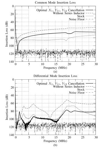
Fig. 17. Performance comparison of the commercially-available EMI filter in Fig. 14 and the modified version in Fig. 15, showing performance both without and with inductance compensation.
