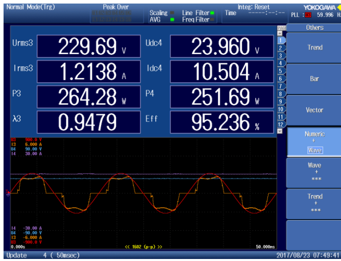
Fig. 8 Line voltage (red), line current (yellow), output voltage (blue) and output current (purple) for the following operating point: 230 Vac input, 24 Vdc output voltage at an output power of 251 W. The power factor is 0.948 and efficiency 95.2%. The converter does not draw peak current when the voltage is maximum. THD i =24%
