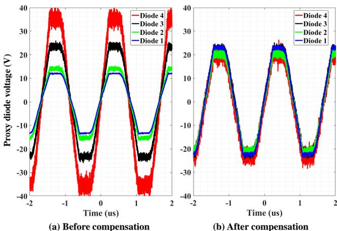
**Figure 9:** Proxy (divided down and ac coupled) diode voltages before/after compensation. In both cases, the rectifier operates at 600 kHz and outputs 3.6 kV 20 mA (72 W). The voltage ratio is 1 : 1.16 : 1.94 : 2.91 before compensation, and 1 : 0.89 : 0.97 : 0.87 after compensation. The worst-case voltage discrepancy as a percentage is  $2.91/1 = 291\%$  and  $1/0.87 = 115\%$ .
