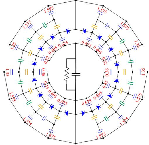
**Figure 14:** The simulated capacitance matrix of the PCB layout in Fig. 13. All capacitances to common (GND or  $V_o$ ) are in red and in pF. The capacitors in green are between two probe pads and are 0.002 pF; the capacitors in yellow are between each diode pad and probe pad and are 0.045 pF
