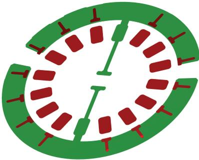
**Figure 13:** The copper layout of the full-bridge rectifier. In the Fast Field Solver [26], one can define a group of conductors (traces, pads, via, etc) as one node. In this geometry, ground node and  $V_o$  node are in green; rest of the nodes are in red. The square-shape pads are nodes connecting two diodes and the T-shape pads are nodes connecting to the probe adapters.
