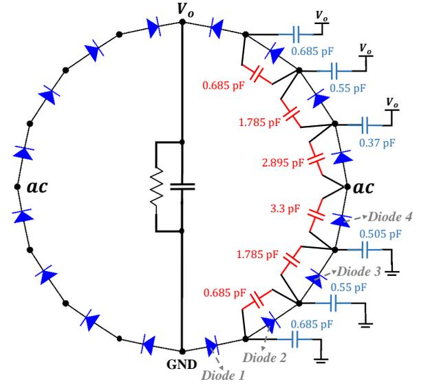
**Figure 7:** The estimated parasitic capacitance of each node to common (in blue) and the required compensation capacitance across each diode (in red). The capacitances are symmetric across the  $V_o$ -GND axis. We implement these using the available capacitors with the closest available capacitance values.
