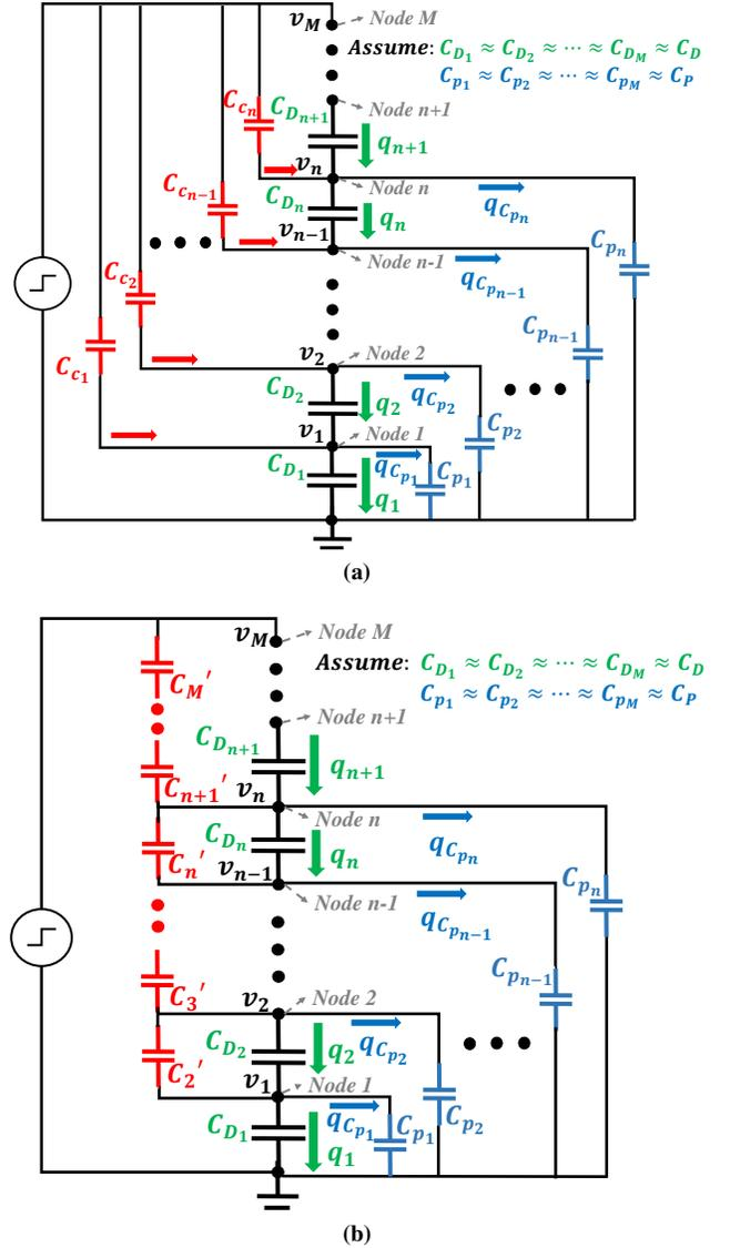
**Figure 4:** Circuit diagram of two related compensation techniques (a) Independent compensation: adding compensation capacitors to each node. (b) Coupled compensation: adding compensation capacitors across each diode.
