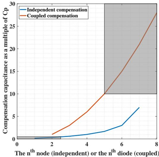
**Figure 5:** Compensation capacitance required at each node normalized to parasitic capacitance  $C_P$ . The compensation capacitance required at any node should not be too small, as limited by the physically realizable capacitance, nor too big, as limited by the physical capacitor size and parasitics. These limits are conceptually illustrated by the two grey areas.
