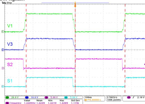
Fig. 9. Experimental waveforms at half load. Compared with the full-power case (Fig. 8), the primary and secondary switches still achieve ZVS (red dashed lines) even though the same control signals are used.
