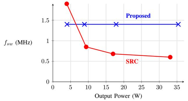
Fig. 12. Simulated switching frequency  $f_{sw}$  of the proposed converter and the SRC, contrasting the constant timing operation of the proposed converter with the variable-frequency nature of the SRC.
