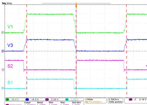
Fig. 8. Experimental waveforms at full load. The primary and secondary switches achieve ZVS (red dashed lines) at the same time using the same control signals.
