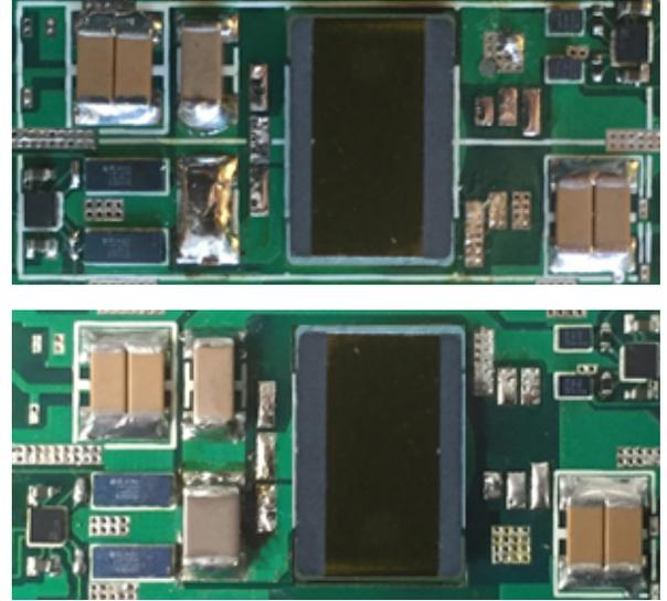
Fig. 5. Top and bottom sides of the prototype converter. The main power stage has a size of 1.2 in  $\times$  0.6 in  $\times$  0.17 in, yielding a power density of 300 W/in<sup>3</sup>.
