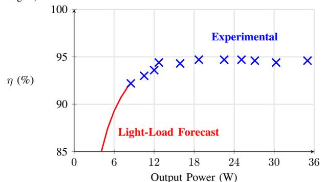
Fig. 11. Experimental efficiency of the prototype converter across power, showing high efficiency for a wide load range since ZVS is maintained; constant magnetizing current causes efficiency droop at light load, which is forecast to lighter-load conditions by assuming constant loss.
