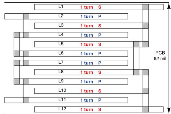
Fig. 6. Transformer layer configuration of the prototype converter. The primary winding has 6 turns, each on a separate layer (94 mil traces). The secondary winding has 2 turns, each formed of 3 parallel traces on separate layers. All windings are realized with 2 oz copper.
