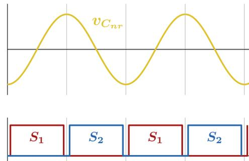
Fig. 7. Expected waveforms when the resonant frequency and operating frequency are properly tuned. The resonant tank can be tuned by measuring the phase of the resonant capacitor voltage referenced to the control signals.
