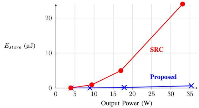
Fig. 16. Simulated resonant energy storage (which corresponds to volume of the resonant elements), contrasting the high energy storage of the SRC (due to its high  $Z_0$  requirement) as opposed to the proposed converter.
