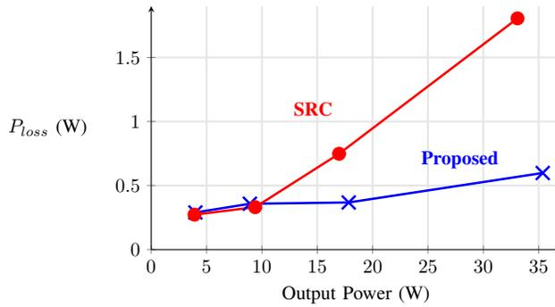
Fig. 15. Simulated losses corresponding to the efficiencies in Fig. 14, highlighting that the volume-setting peak losses in the SRC are significantly higher than in the proposed converter.
