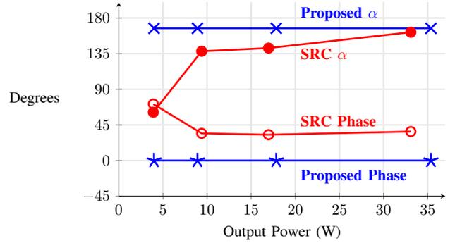
Fig. 13. Simulated conduction angle  $\alpha$  and phase shift of the secondary switches to achieve ZVS with minimal diode conduction, contrasting the load-invariant operation of the proposed converter with the highly load-dependent operation of the SRC. Because the SRC depends upon the resonant current to achieve ZVS, the conduction angle decreases with load, which also causes losses without transferring power.
