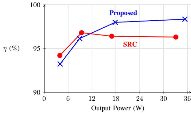
Fig. 14. Simulated efficiency for the proposed converter, showing comparable light-load behavior with greatly improved full-load efficiency for the proposed converter.
