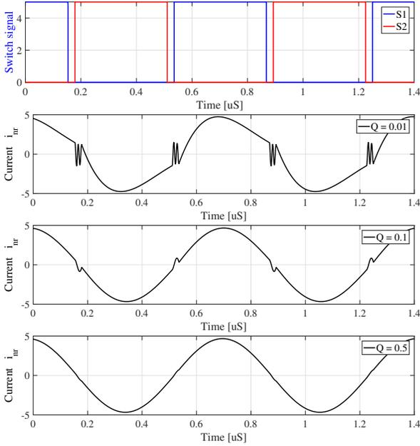
Fig. 4. Simulated resonant tank currents for various quality factors. Quality factors as low as 0.1 yield near-ideal resonant current.
