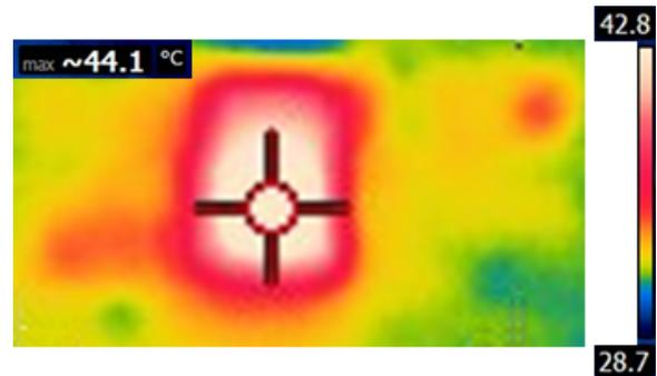
Fig. 10. Infrared thermal image of the converter operating at full power in a  $25^\circ\text{C}$  ambient without active cooling. Low temperature rise is achieved and low switch losses in particular are expected from achieving ZVS (compare to Fig. 5).
