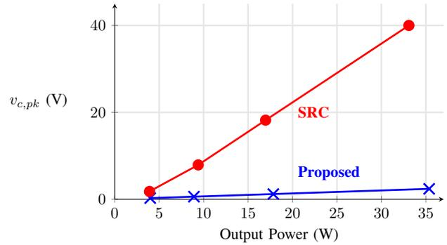
Fig. 17. Simulated peak resonant capacitor voltages (which may set spacing and part availability for some applications), contrasting the high voltages in the SRC (due to its high  $Z_0$  requirement) as opposed to the proposed converter.
