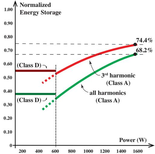
Fig. 9. Class D regulation limits do not seamlessly transition into their Class A maxima at 600 W, hence the discontinuity in achievable energy storage at this boundary. Almost two-thirds of the possible energy storage reduction across a wide range of power can be achieved through the 3rd harmonic alone.
