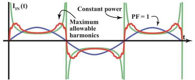
Fig. 3. Input current waveforms for PF = 1 (blue), zero-buffer solution (green), and maximum Class D harmonic current (red). The maximum harmonic current waveform closely approximates the zero-buffer current for a large portion of line cycle.
