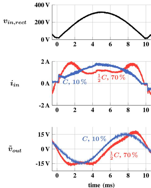
Fig. 16. Comparison of output voltage ripple when harmonics are included (10% vs 70% of the allowable third and fifth harmonics) and capacitance is reduced. The reduced voltage ripple of about 50% in Fig. 14 is traded for 50% less capacitance.
