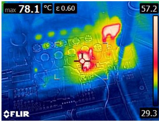
Fig. 18. Thermal capture of the converter operating with 70% of allowable harmonics, showing that diode losses (which are harmonic-independent) dominate in this prototype. The hot spot in the center is the boost diode, and the hot spot in the upper right is the diode bridge.
