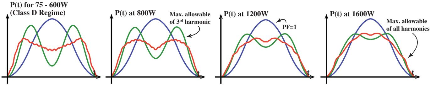
Fig. 8. Power waveforms when including all available harmonic currents are identical across the 75 W-600 W Class D range. Beyond 600 W (in Class A), the benefits brought by harmonic currents diminishes as their relative weight to the fundamental decreases. Still, this method yields up to a 35% reduction in energy storage at 1600 W.
