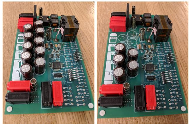
Fig. 15. Photograph of prototype PFC showing the available buffer size reduction when introducing 70% of third and fifth harmonic Class D limits with constant output ripple. The capacitor reduction matches theory, and is a major improvement to the system power density.
