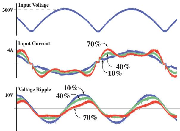
Fig. 13. Experimental input voltage, input current, and output voltage ripple for 10% (blue), 40% (yellow), and 70% (purple) of the allowed 3rd and 5th harmonic. The output voltage ripple decreases for fixed capacitance, as expected; the original voltage ripple could be restored with less capacitance and improved power density.
