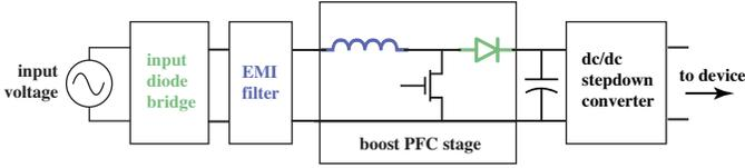
Fig. 10. The two-stage converter with boost PFC is a very popular grid-interface architecture. For this example, incorporating input current harmonics may negatively impact losses in the diode bridge, EMI filter, and boost inductor, should not affect the boost diode or dc/dc step-down converter, and may improve losses in the buffer capacitor and boost switch.
