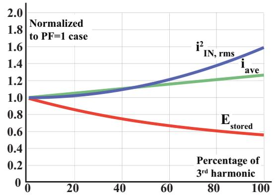
Fig. 12. Increases in  $i_{in,ave}$  and  $i_{in,rms}$  for a given energy storage reduction goal when using only allowable third harmonic.
