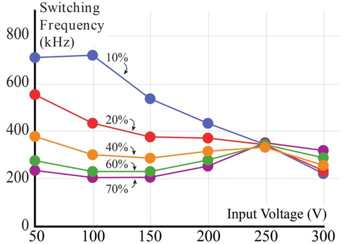
Fig. 19. Local operating frequency of the valley-switched boost PFC across the first half of the rectified input voltage half-cycle. The variable frequency introduced by the valley-switched boost is greatly mitigated with the inclusion of input harmonics, by drawing more current at low voltage.
