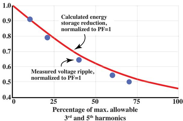
Fig. 14. Experimental output voltage ripple, normalized to the PF = 1 case, showing a close match to theory.
