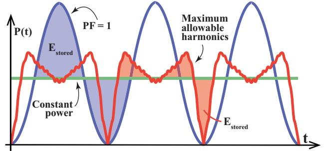
Fig. 4. The energy storage requirement when using maximum allowable Class D harmonics (shaded area, red) is significantly decreased from the energy storage required at PF = 1 (shaded area, blue).
