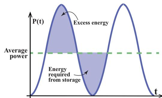
Fig. 2. When  $PF = 1$ , power oscillates  $\propto \sin^2$ ; integrating over time relative to average (desired) power gives energy storage requirement over a line cycle, shown as shaded.
