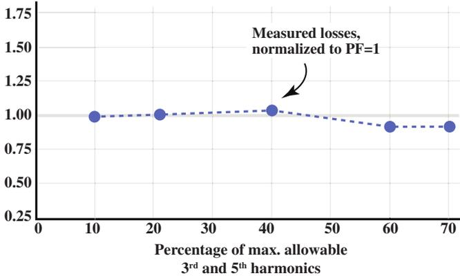
Fig. 17. Measured converter losses, normalized to the low-harmonic case (10% harmonic usage, 96% efficiency). In this prototype, which is dominated by diode losses, including significant harmonic content has negligible effect on efficiency.
