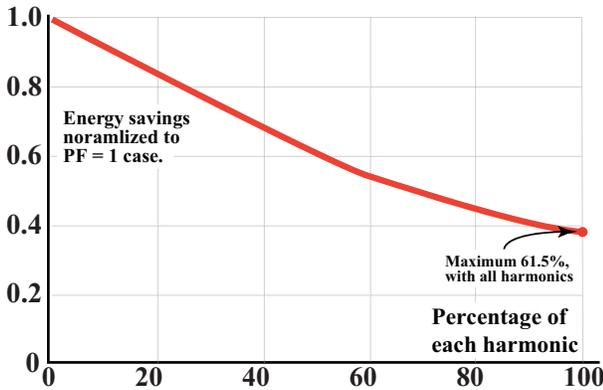
Fig. 5. Energy storage requirement as all harmonics are included at the same percentage  $p$  of their individual allowed maxima under Class D. By including all every available harmonic, the energy storage requirement can be reduced by nearly 62%
