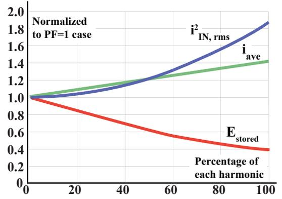
Fig. 11. Increases in  $i_{in,ave}$  and  $i_{in,rms}$  for a given energy storage reduction goal when using all allowable harmonic currents at equal percentages relative to their EN61000-3-2 limits.
