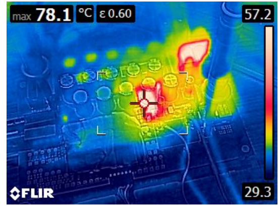
Fig. 26. Thermal capture of the converter operating with 70 % of allowable harmonics, showing that diode losses (which are harmonic-independent) dominate in this prototype. The hot spot in the center is the boost diode, and the hot spot in the upper right is the diode bridge.
