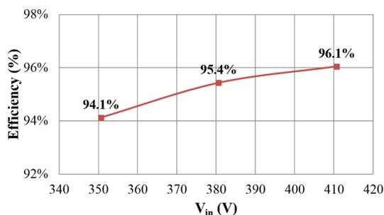
Fig. 23. Experimental efficiency of the Si DSAB converter delivering 300 W over an input voltage range of 350 V to 410 V.
