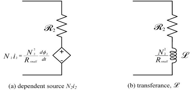
Fig. 10. (a) A model of the shorted winding (here, shown as winding 2), represented as a dependent source that produces a current  $i_2$  to effectively cancel all flux in that leg. Nonidealities such as path resistance are represented by some small resistance  $R_{small}$ . (b) Equivalent transference model for the shorted winding, modeling it with some transference,  $\mathcal{L} = (N_2)^2/R_{small}$ .
