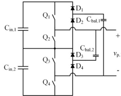
Fig. 19. Balancer circuit used to balance the input capacitors within one stacked full-bridge inverter.  $C_{in,1}$  and  $C_{in,2}$  are balanced with respect to each other using  $C_{bal,1}$  and  $C_{bal,2}$ . Only the top inverter, connected to  $V_{inv,1}$  is shown here; the same circuit is used on the bottom inverter. Values for the balancer components are given in Table III.
