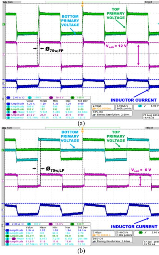
Fig. 20. Operating waveforms for the GaN DSAB converter with an input voltage of 380 V, an output voltage of 12 V, and an output power of 75 W in (a) full-power mode at a phase shift of  $8.1^\circ$  (0.141 rad), and (b) low-power mode at a phase shift of  $18.0^\circ$  (0.314 rad).
