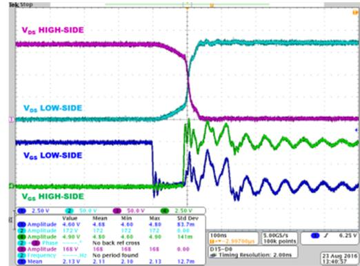
Fig. 22.  $V_{ds}$  and  $V_{gs}$  waveforms for an inverter half-bridge in the Si single-stacked DAB converter operating with an input voltage of 380 V, an output voltage of 12 V, and a phase shift of  $14.7^\circ$  (0.257 rad) to deliver 150 W. The switches are hard-switched for most of the switch transition.
