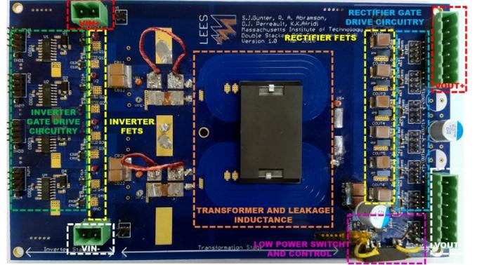
Fig. 15. Top side of the GaN-based DSAB prototype. The inverter and rectifier devices and control circuitry are labeled, as is the single-core magnetic component.
