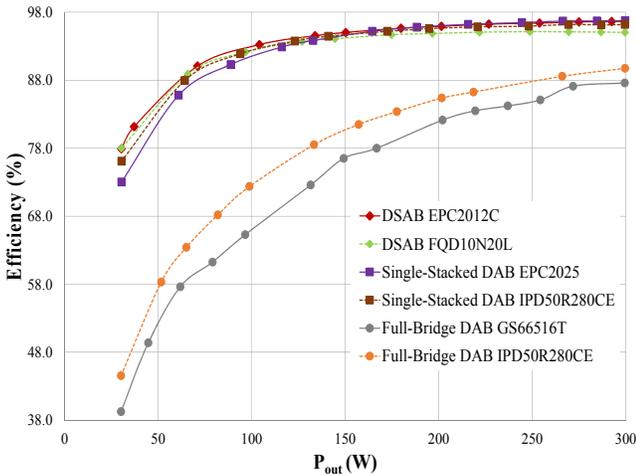
Fig. 13. Simulated efficiency curves for all topologies with all device combinations. The full-bridge DAB converter (shown in orange and gray), has much lower efficiency across the entire power range compared to the stacked topologies. While the single-stacked DAB has similar efficiencies to that of the DSAB at full-power, it becomes much less efficient with decreasing output power, due to losing ZVS earlier than the DSAB converter.
