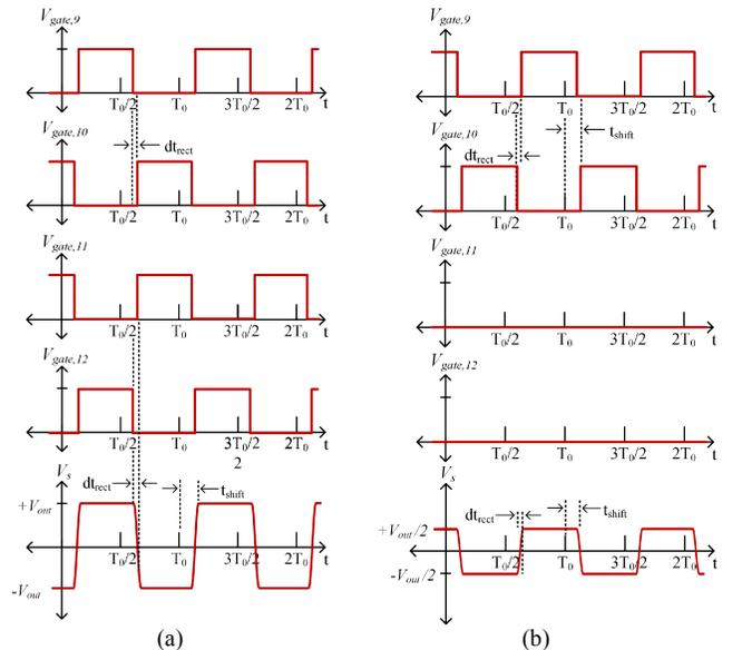
Fig. 7. Switching diagram for the rectifier secondary voltage, while the converter is operating in (a) full-power mode and (b) low-power mode.
