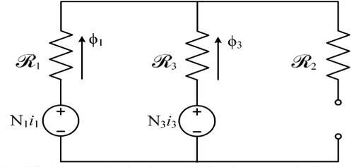
Fig. 9. Simplified magnetic circuit model for the three-winding transformer operating in the low-power mode, for the case when primary winding 2 is held at zero voltage, by connecting an ac short across it. Let  $N_1 = N$  and  $N_3 = 1$ .
