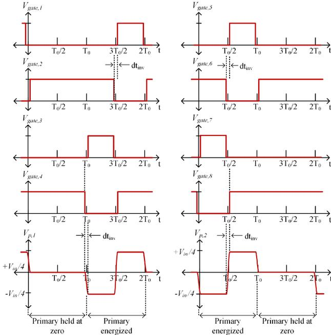
Fig. 8. Switching diagram for the inverter and primary winding voltages, while the converter is operating in the low-power mode.
