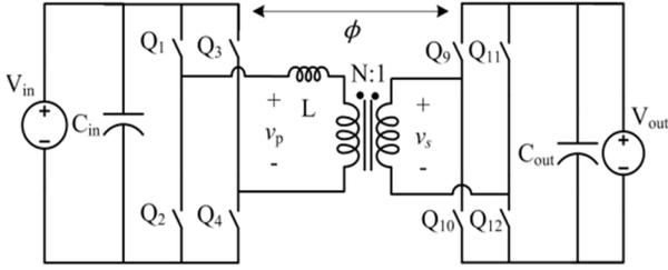
Fig. 1. A DAB converter with a full-bridge input and output. The two bridges are phase-shifted from each other across a transformer and an inductance,  $L$ .
