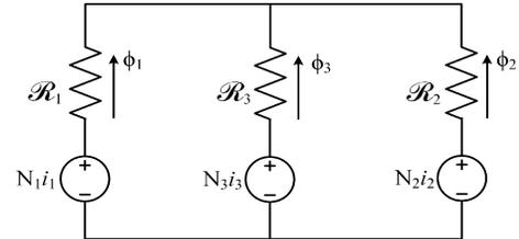
Fig. 5. A magnetic circuit model for the three-winding transformer.  $N_1i_1$ ,  $N_2i_2$ , and  $N_3i_3$  represent the magnetomotive forces of each winding, while  $\mathcal{R}_1$ ,  $\mathcal{R}_2$ , and  $\mathcal{R}_3$  represent the reluctances of the core for each leg.
