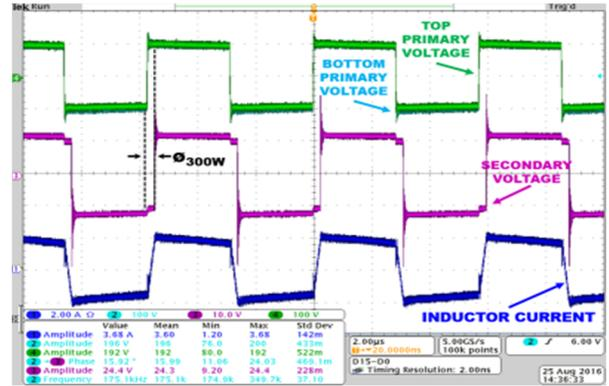
Fig. 18. Operating waveforms for the GaN DSAB converter operating in full-power mode with an input voltage of 380 V, an output voltage of 12 V, and a phase shift of  $17.2^\circ$  to deliver 300 W (100% load).
