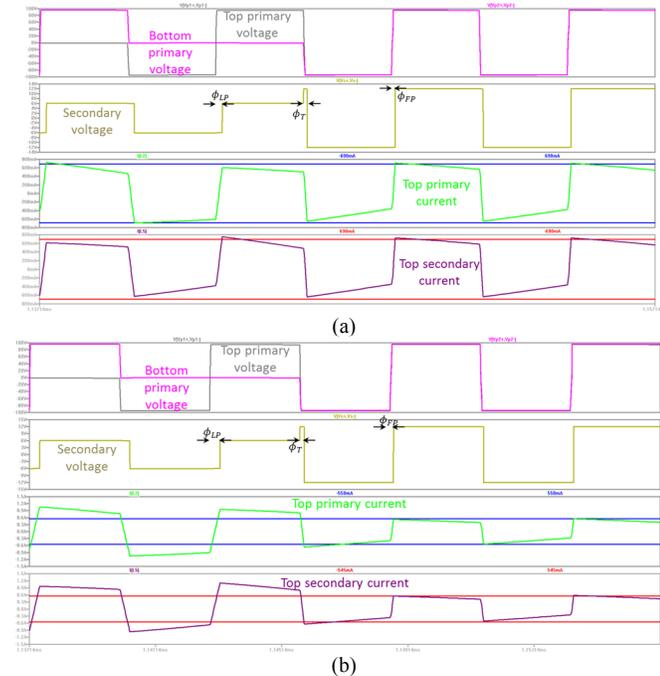
Fig. 29. Zoomed in simulated operating waveforms for the GaN DSAB converter for (a) a transition from the full-power mode to low-power mode, while maintaining the output power at 75 W across the mode-switch, and (b) a transition from the full-power mode to low-power mode for a step in output power from 100 W to 50 W. The full-power phase-shift  $\phi_{FP}$ , low-power phase-shift  $\phi_{LP}$ , and transition phase-shift  $\phi_T$ , are labeled.
