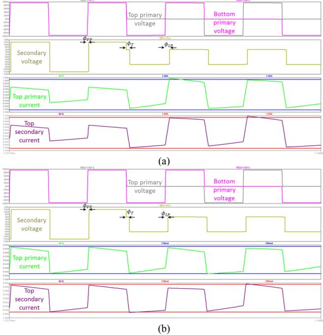
Fig. 27. Zoomed in simulated operating waveforms for the GaN DSAB converter for (a) a transition from low-power to full-power mode, while remaining at 75 W, and (b) a transition from low-power to full-power mode for a step in output power from 100 W to 50 W. The full-power phase-shift  $\theta_{FP}$ , low-power phase-shift  $\theta_{LP}$ , and transition phase-shift  $\theta_T$ , are labeled.
