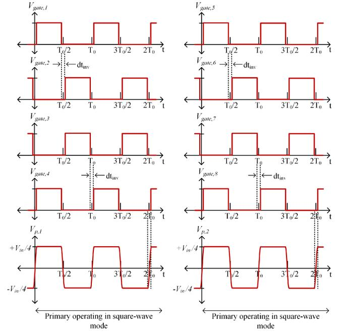
Fig. 6. Switching diagram for the inverter and primary winding voltages, while the converter is operating in the full-power mode.
