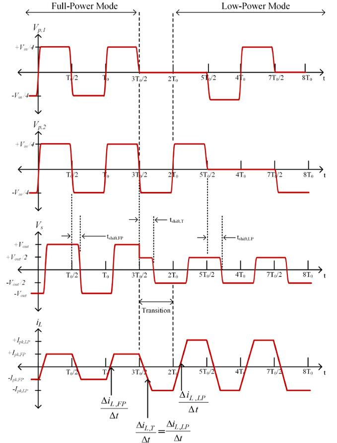
Fig. 11. Converter primary and secondary winding voltages and leakage inductor current, during a mode switch from the full-power mode to the low-power mode. The slopes of the inductor current waveform are labeled.
