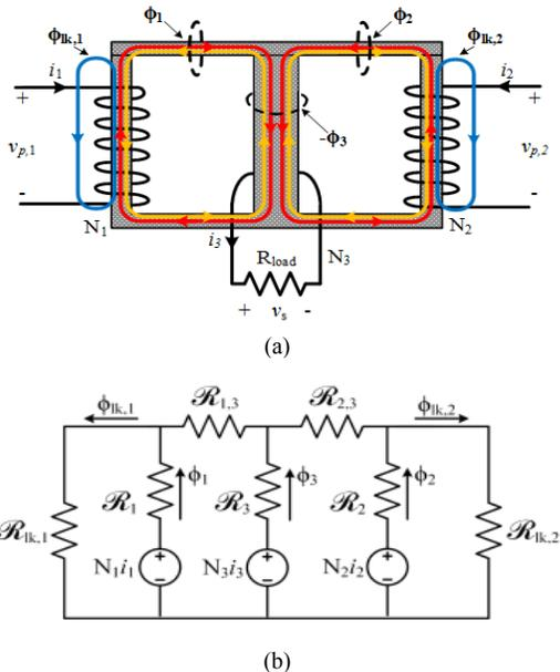
Fig. 17. (a) Diagram of the flux paths of the three-winding transformer. Fluxes  $\phi_1$  and  $\phi_2$  in the outer legs link the secondary, and  $-\phi_3$  is the flux through the center leg. Fluxes  $\phi_{1k,1}$  and  $\phi_{1k,2}$  are the primary winding leakage fluxes that do not link to the secondary. (b) The equivalent magnetic circuit model that includes the primary-side leakage paths, as well as the main flux paths through the core legs.
