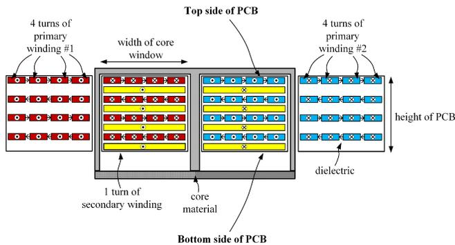
Fig. 16. Cross-section of the magnetic core and PCB layer stack-up for the three-winding transformer. The red and light blue primary windings are interleaved inside the core window with the yellow secondary windings.
