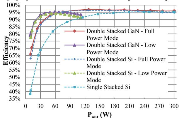
Fig. 25. Experimental efficiency curves across output power for double stacked converters populated with GaN and Si switches operating in full power and low-power modes, as well as a curve for a single stacked converter with Superjunction Si switches.
