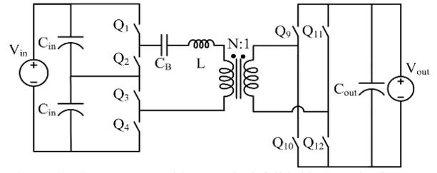
Fig. 3. A DAB converter with a stacked full-bridge on the input and a full-bridge on the output. A blocking cap,  $C_B$ , is used to remove the DC component in the square-wave output of the stacked-bridge.
