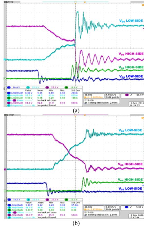
Fig. 21.  $V_{ds}$  and  $V_{gs}$  waveforms for an inverter half-bridge in the GaN DSAB converter operating at 75 W in (a) the full-power mode and (b) the low power mode. The low-power mode is able to mostly achieve soft-switching, while the full-power mode experiences substantial hard-switching.
