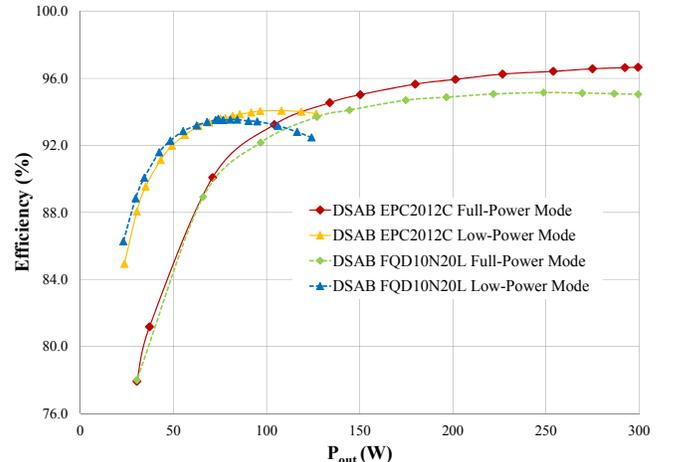
Fig. 14. Simulated efficiency curves for the Si and GaN DSAB converters operating in the full-power and low-power modes.
