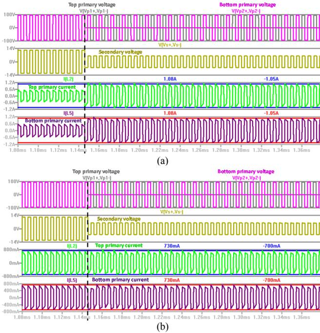
Fig. 26. Simulated operating waveforms for the GaN DSAB converter for (a) a transition from the full-power mode to low-power mode at a constant 75 W, and (b) a transition from the full-power mode to low-power mode for a step in output power from 100 W to 50 W. The blue and red sets of horizontal lines show the steady-state amplitude of the current.
