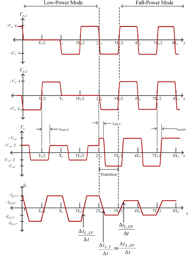
Fig. 12. Converter primary and secondary winding voltages and inductor current, during a mode switch from the low-power mode to the full-power mode. The slopes of the inductor current waveform are labeled.
