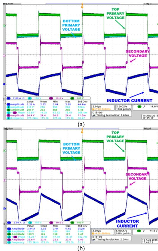
Fig. 24. Si DSAB converter operating waveforms at an input voltage of (a) 410 V and (b) 350 V, both at an output voltage of 12 V and an output power of 300 W.
