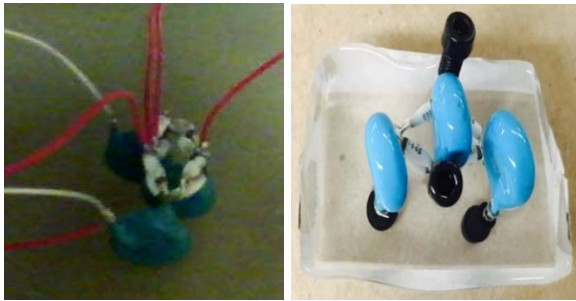
Fig. 10 Air-insulation (left) and PDMS insulation (right)
