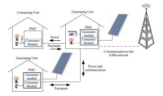
Figure 1: The Power Management Units (PMUs) can connect generating sources, batteries and loads to form an ad-hoc dc microgrid with peer-to-peer electricity sharing.
