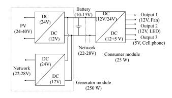
Figure 5: A possible network architecture with cascaded converters and direct battery voltage distribution.
