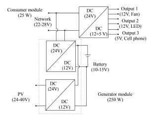
Figure 6: A possible network architecture with parallel converters.
