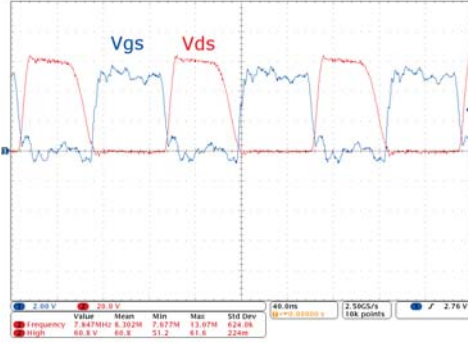
Fig. 12. Experimental v_{gs} and v_{ds} waveforms showing zero-voltage switching of the HF regulation stage (x: 40ns/div, y- v_{gs} : 2V/div, y- v_{ds} : 20V/div). The HF stage input voltage is 60 V and the output is a 35 V, 12.15 W load. The converter operates at 7.85 MHz under this condition.
