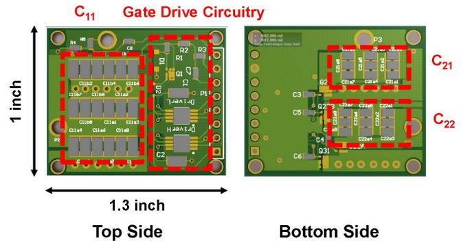
Fig. 10. Composition of the SSC energy buffer PCB, including the  $C_{11}$ ,  $C_{21}$ ,  $C_{22}$  and the gate driver circuitry.
