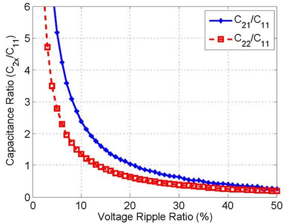
Fig. 6. Optimal capacitance ratios as a function of ripple ratio for the 1-2 enhanced unipolar SSC energy buffer.
