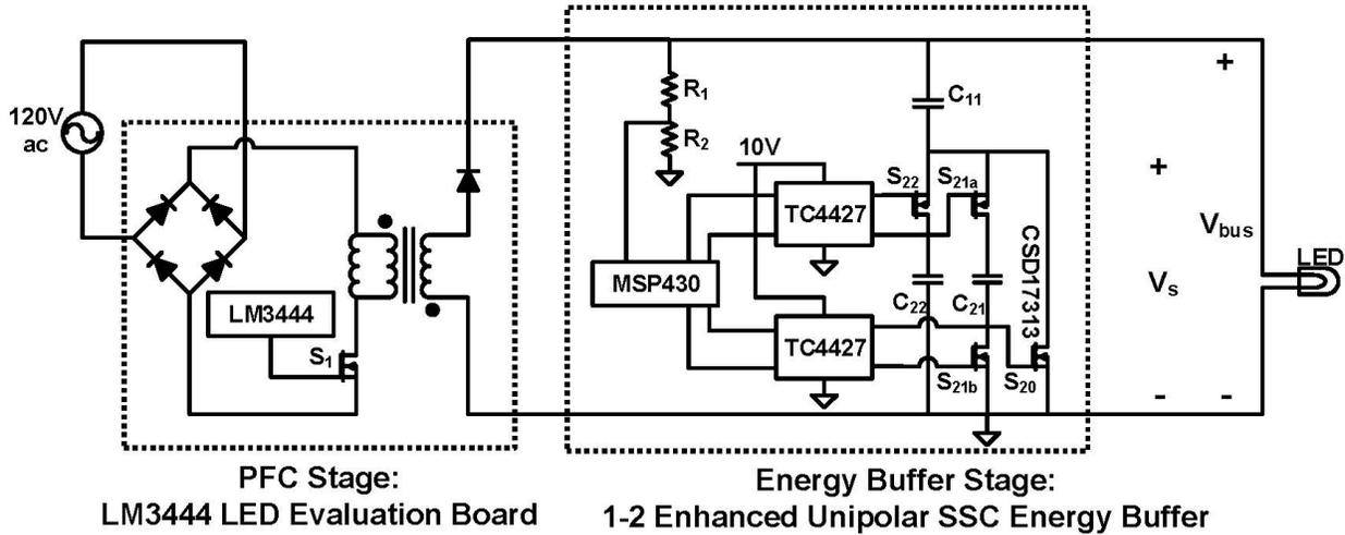
Fig. 8. Switch, gate-drive and control implementation of the prototype SSC energy buffer as part of the offline LED driver.
