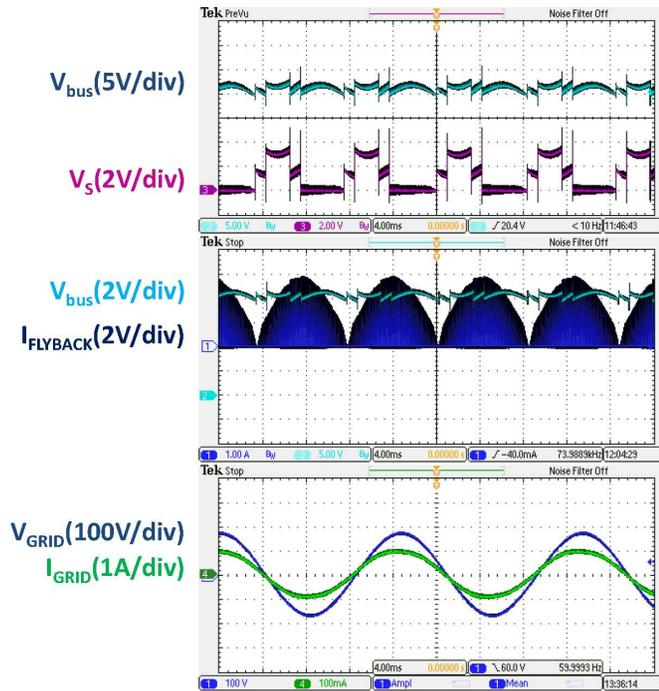
Fig. 11. Measured operation waveforms of the prototype, including the bus voltage  $V_{bus}$ , the voltage at the switch node  $V_s$ , the output current of the flyback converter  $I_{FLYBACK}$ , and the grid current  $I_{GRID}$ .
