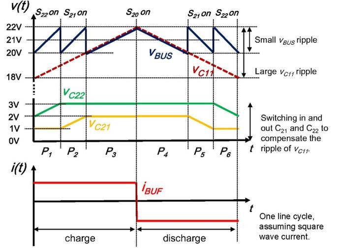
Fig. 3. Operation waveforms of a 1-2 enhanced unipolar SSC energy buffer.
