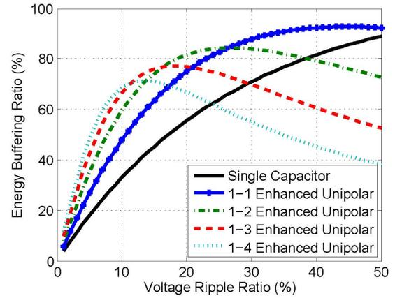
Fig. 4. Energy buffering ratio of the  $1 - m$  enhanced unipolar SSC energy buffer as a function of ripple ratio with different number of supporting capacitors ( $m$ ). The energy buffering ratio for a single capacitor is also shown for comparison.
