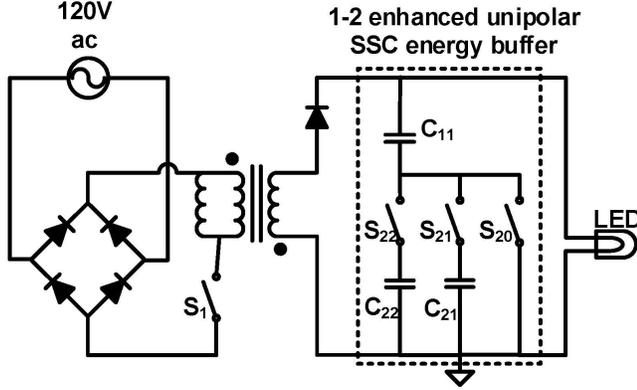
Fig. 2. A 1-2 enhanced unipolar SSC energy buffer as part of an offline single-stage LED driver.
