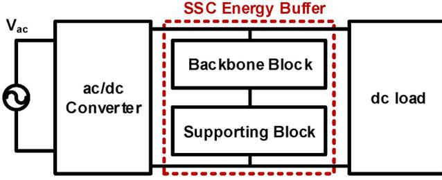
Fig. 1. Stacked Switched Capacitor (SSC) energy buffer architecture.
