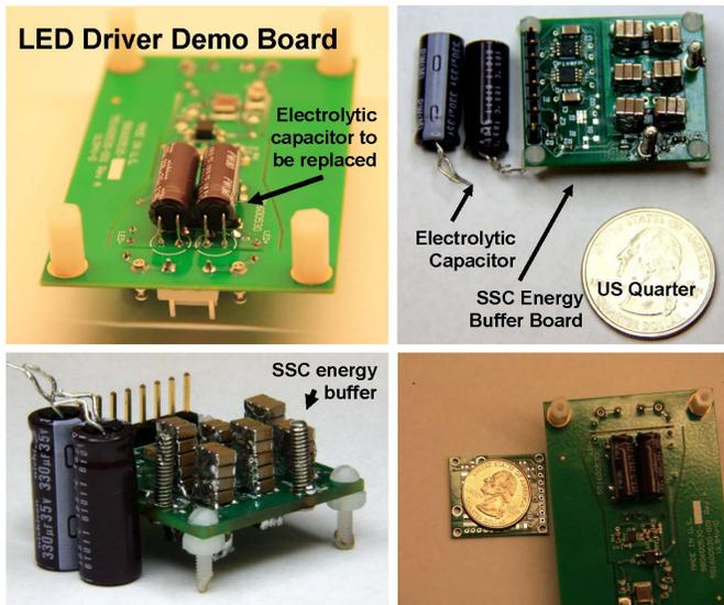
Fig. 9. Photograph comparing the size of the SSC energy buffer to that of the electrolytic capacitors it replaces. Also shown (top) is the LED driver.
