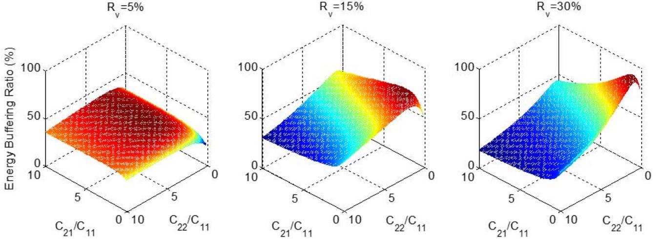
Fig. 5. Energy buffering ratio of a 1-2 enhanced unipolar SSC energy buffer as a function of the ratio of its capacitances ( $\frac{C_{21}}{C_{11}}$  and  $\frac{C_{22}}{C_{11}}$ ) for different ripple ratios ( $R_v$ ): (a)  $R_v = 5\%$ , (b)  $R_v = 15\%$ , and (c)  $R_v = 30\%$ .
