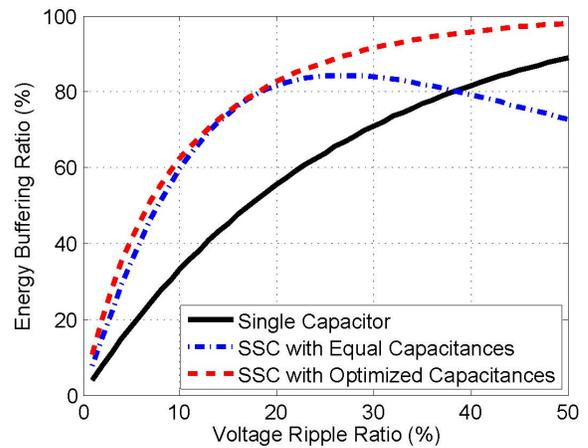
Fig. 7. Improvements of energy buffering ratio due to capacitance ratio optimization in a 1-2 enhanced unipolar SSC energy buffer.
