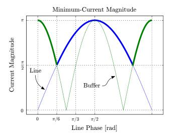
Fig. 8. This illustrates the minimum resonant current magnitude requirements for the buffer-block and cycloconverter, including the bold line indicating the envelope of current that meets both constraints.
