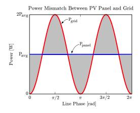
Fig. 1. The power flow mismatch between the grid and a constant power source results in the shaded area, representing the required energy storage.
