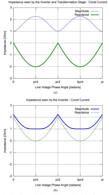
Fig. 12. The normalized load impedance, at the switching frequency, presented to the full-bridge inverter by (a) the buffer-block, and cycloconverter stages, and (b) including the series-resonant tank. Without the inductance of the resonant tank, the reactance presented to the inverter prevents zero-voltage switching.
