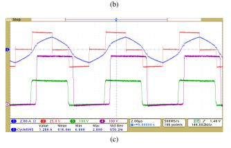
Fig. 15. Converter operation with 32 V input, 100 W average power, at three points in the line cycle: (a) zero degrees, 0 V; (b) 30 degrees, 170 V; (c) 90 degrees, 340 V. Waveform color key; (1) blue: current, (2) red: full-bridge, (3) green: buffer-block, (4) purple: cycloconverter. Channels 1 and 2 are referenced to the top marker, while channels 3 and 4 are referenced to the bottom marker.
