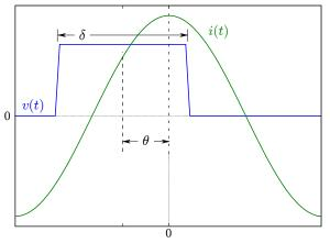
Fig. 7. The current and voltage operating waveforms of the constituent sub-circuit in Fig. 6, illustrating the control parameters  $\delta$  and  $\theta$ .
