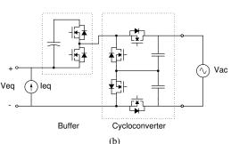
Fig. 5. Equivalent circuits representing the (a) primary and (b) secondary sides, decoupled by approximating the output of the transformation stage as a current source.
