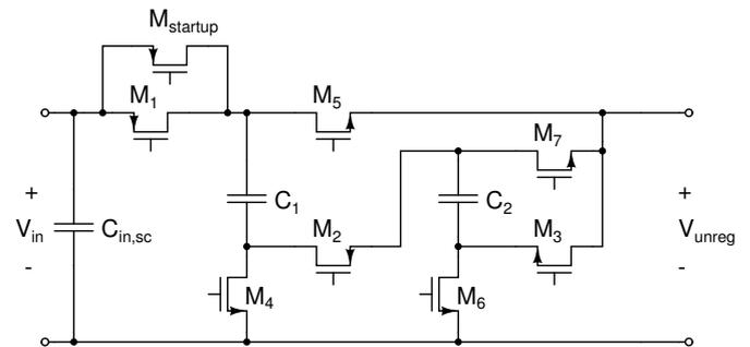
Fig. 6. Schematic drawing of switched-capacitor transformation stage. The capacitors are off-chip, and the transistors are 5 V triple-well thick-oxide devices available in the 180 nm CMOS process.
