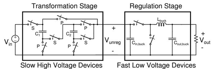
Fig. 1. Block diagram illustrating the two-stage architecture, which enables large voltage step down and high frequency operation on the same die.
