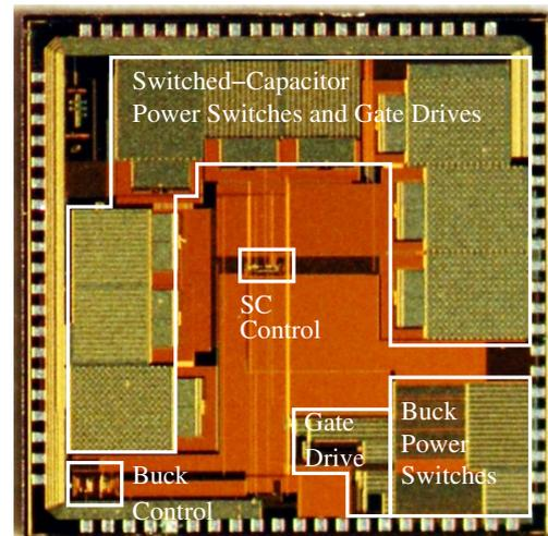
Fig. 7. Die photograph of the converter implemented in 180 nm CMOS technology. The total die area is 5x5 mm, although much of that area is not used.
