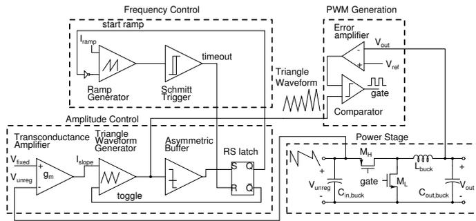
Fig. 5. Block diagram illustrating feed-forward control. The height of the triangle waveform is proportional to the regulation stage input voltage ( $V_{unreg}$ ).
