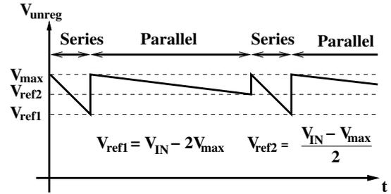
Fig. 3. Ideal waveforms illustrating the switched-capacitor control strategy to maintain the SC stage output voltage below  $V_{max}$ , thus enabling the use of low-voltage devices in the regulation stage.
