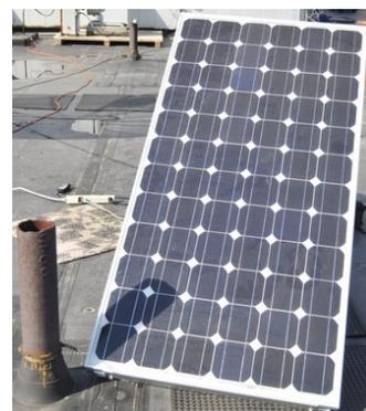
Fig. 7. Photograph illustrating the shading (owing to a protruding pipe) that moves across the module for the dynamic performance experiment.
