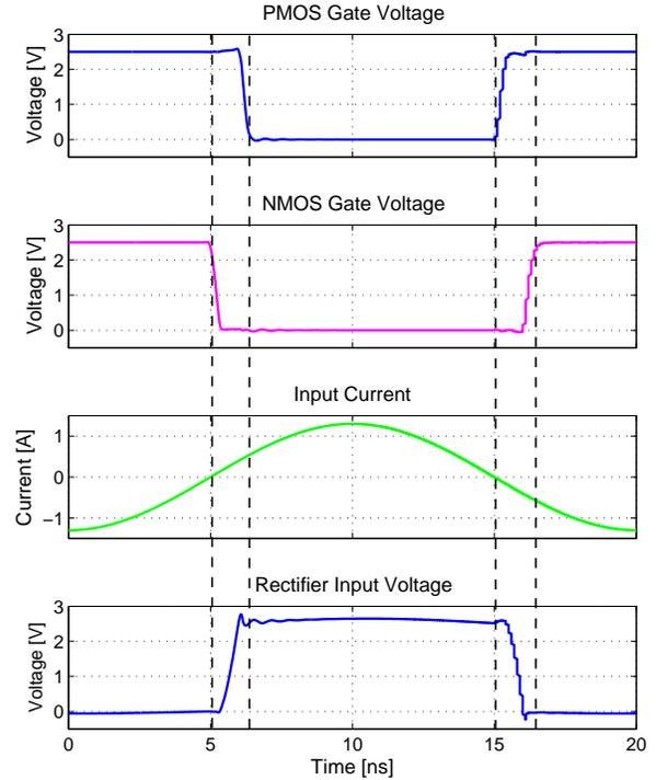
Fig. 11. Simulated soft-switched class D rectifier switching waveforms. It shows that both devices can achieve zero-voltage turn-on and close to zero-current turn off.
