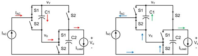
Fig. 6. Switching patterns of the switched-capacitor rectifier.
