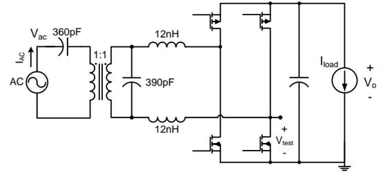
(a) Full-bridge rectifier schematic
