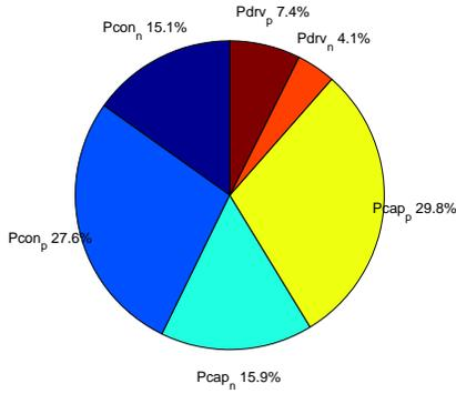
Fig. 10. Figure shows the loss break down in the rectifier.  $P_{con_n}$  and  $P_{con_p}$  mean the conduction loss in NMOS device and PMOS device respectively,  $P_{cap_n}$  and  $P_{cap_p}$  are the capacitively loss for the NMOS device and PMOS device.  $P_{drv_n}$  and  $P_{drv_p}$  are the gate driver loss for the devices.
