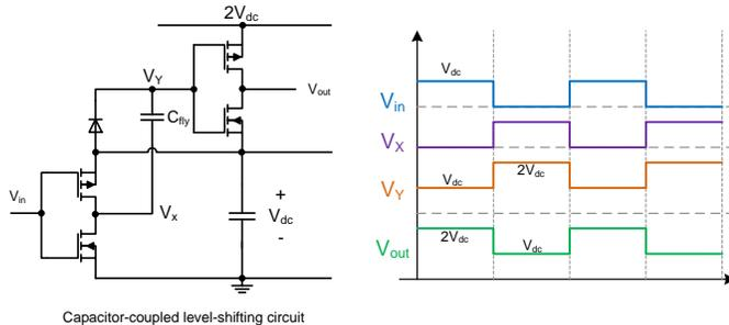
Fig. 14. The schematic of the level shifting circuit.
