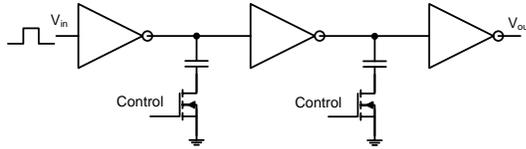
Fig. 13. The schematic of the voltage-controlled delay line.
