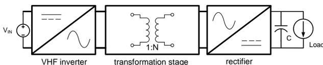
Fig. 1. A architecture for a dc-dc converter.
