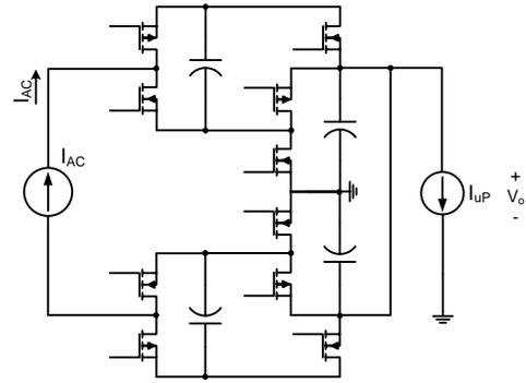
Fig. 9. Schematic of a double-ended two-step switched-capacitor rectifier.
