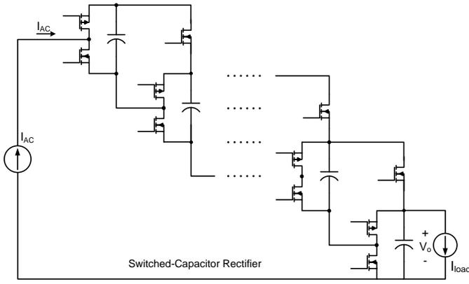
Fig. 3. General schematic of a multi-step switched-capacitor rectifier.
