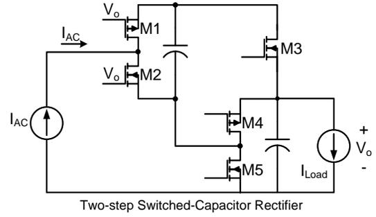
Fig. 4. Sample schematic of a two-step CMOS switched-capacitor step-down rectifier. The drive and control structure is shown in Fig. 5. Note that in some cases a dc blocking capacitor (not shown) may be desired at the rectifier input; this does not change the rectification characteristics.
