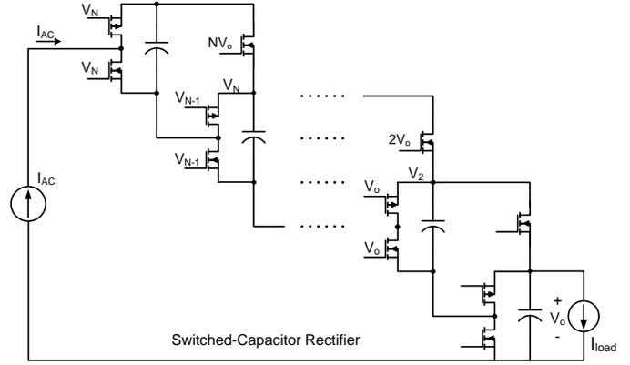
Fig. 8. Self-driven scheme for the multi-level switched-capacitor rectifier circuit.
