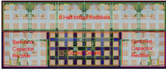
(a) Layout of the rectifier chip
