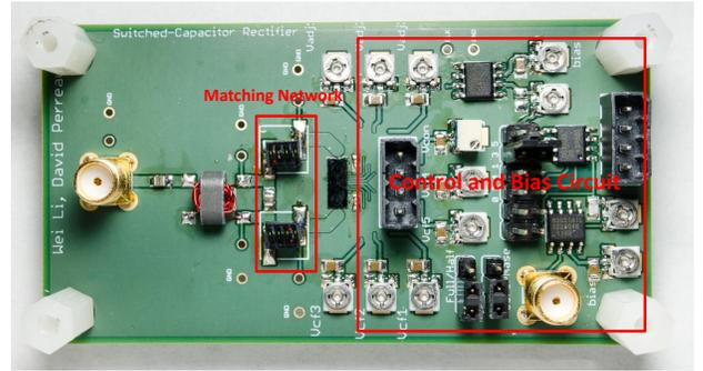
Fig. 17. A picture of the switched-capacitor rectifier prototype board. The black rectangle in the middle of the board is the rectifier IC.
