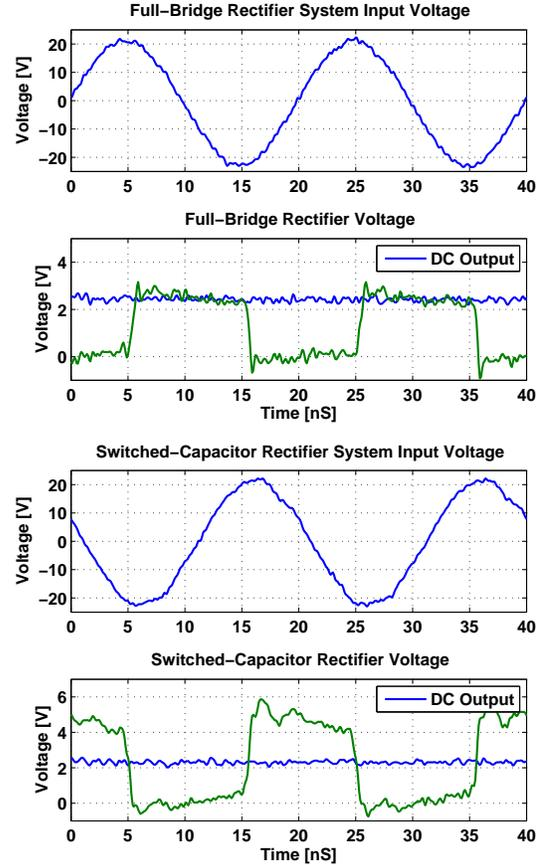
Fig. 19. Experimental waveforms of the rectifier prototypes. Only one phase of the full-bridge rectifier input voltage is shown here, which is ground referenced. The other phase of the rectifier input voltage is simply shifted by a half cycle from the waveform shown here.
