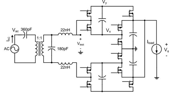
(b) Double-ended SC rectifier schematic
