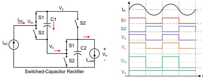
Fig. 7. Switched-capacitor rectifier operating waveforms.
