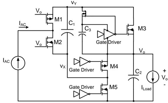
Fig. 5. Control details of the switched-capacitor rectifier.
