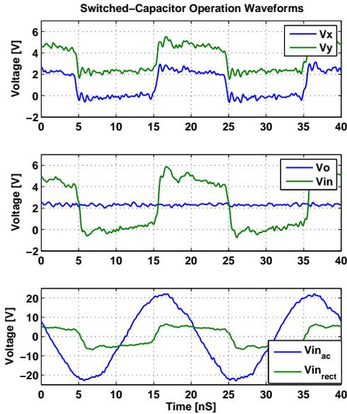
Fig. 18. Experimental waveforms show the operation of the double-ended switched-capacitor rectifier.
