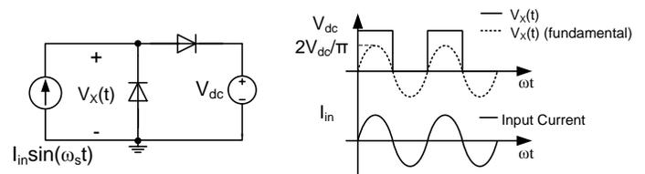
Fig. 2. The half-bridge rectifier and its characteristics. When provided with a dc blocking capacitor at its input, this design can also be recognized as a "voltage doubler" rectifier.
