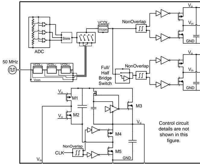
Fig. 12. A simplified schematic of the chip. Control circuit details are not shown in the figure. In addition, only a single full-bridge rectifier and single-ended switched-capacitor rectifier are shown.  $VCDL_c$  is the coarse control of the voltage-controlled delay line and  $VCDL_f$  is the fine-tune control of the voltage-controlled delay line.
