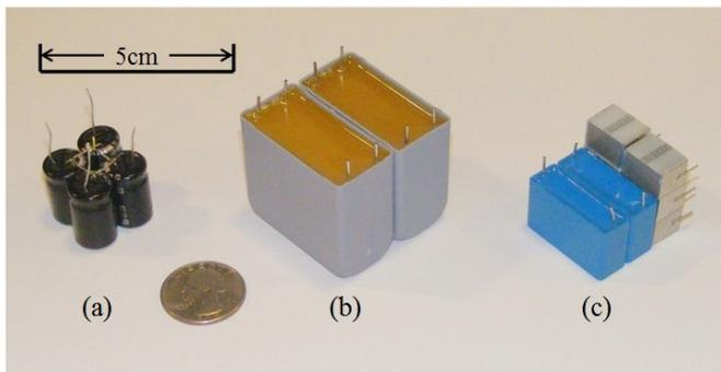
Fig. 14: Relative size of passive energy storage components in different energy buffer architectures: (a) electrolytic-capacitor-only ( $9 \text{ cm}^3$ ) (b) film-capacitor-only ( $65 \text{ cm}^3$ ) and (c) film-capacitor-based SSC ( $20 \text{ cm}^3$ ) energy buffer.
