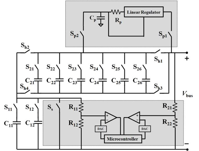
Fig. 9: Precharge circuit (shaded regions) for the 2-6 bipolar SSC energy buffer.
