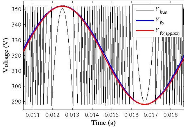
Fig. 11: Comparisons between the accurate ( $V_{fb}$ ) and approximate ( $V_{fb(\text{approx})}$ ) artificial feedback voltages for a sinusoidal energy buffer terminal current.
