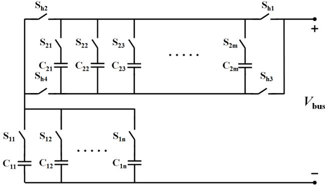
Fig. 6: The  $n$ - $m$  bipolar SSC energy buffer. The circuit has  $n$  backbone capacitors,  $m$  supporting capacitors and  $(n+m+4)$  switches.
