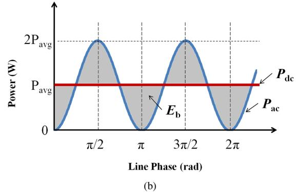
Fig. 1: Mismatch in instantaneous power between single-phase ac,  $P_{ac}$ , and constant power dc,  $P_{dc}$ , results in the need for an energy buffer, as shown in (a), to absorb and supply the energy,  $E_b$ , indicated by the shaded area in (b).
