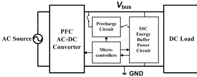
Fig. 8: Block diagram of the prototype setup consisting of a power factor correction (PFC) ac-dc converter, a dc load and the prototyped SSC energy buffer. The prototyped SSC energy buffer consists of: the SSC energy buffer power circuit, the precharge circuit, and the control unit.
