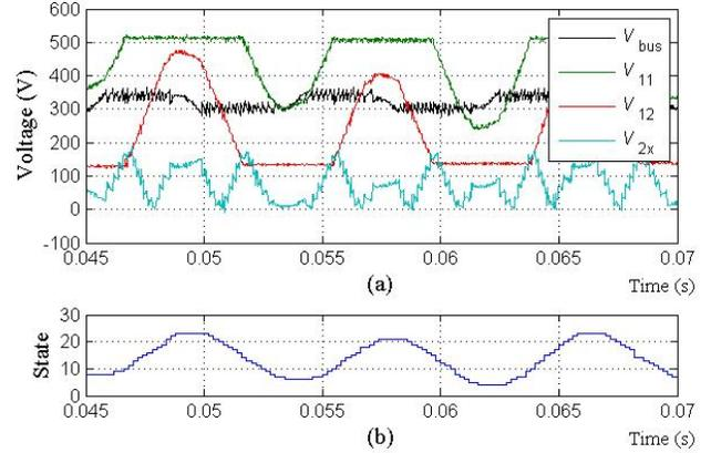
Fig. 12: Measured waveforms of (a) bus voltage ( $V_{\text{bus}}$ ), backbone capacitor voltages ( $V_{11}$  and  $V_{12}$ ) and voltage across the supporting capacitor that is charging or discharging at the time ( $V_{2x}$ ), and (b) corresponding state (1-24) of the state machine.
