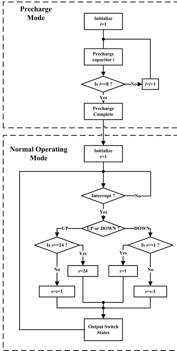
Fig. 10: Flow chart showing the control logic during precharge and normal operation of the 2-6 bipolar SSC energy buffer.
