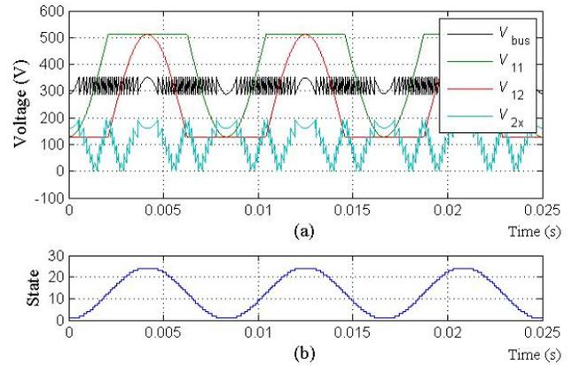
Fig. 13: Simulated waveforms of (a) bus voltage ( $V_{\text{bus}}$ ), backbone capacitor voltages ( $V_{11}$  and  $V_{12}$ ) and voltage across the supporting capacitor that is charging or discharging at the time ( $V_{2x}$ ), and (b) corresponding state (1-24) of the state machine.
