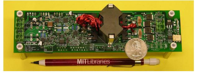
Fig. 8. Photograph of the prototype MEB micro-inverter. Also shown are a pencil and a US quarter to indicate relative size.
